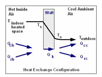
When one side of the wall is warmer than the other side, heat will conduct from the warm side into the material and gradually move through it to the colder side. A temperature gradient is established across the thickness of the wall. The temperature gradient is linear between the two surfaces for a homogenous wall and the slope of temperature gradient is proportional to the resistances of individual layers for a composite structure.
